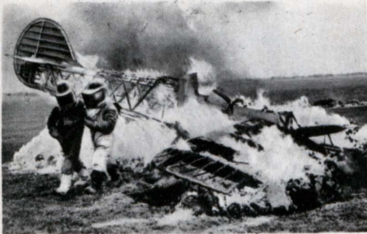
Not until the blazing airplane in which he was testing an asbestos suit was almost reduced to ashes did this inventor, shown at right, leave the cockpit. He was unharmed by heat.
