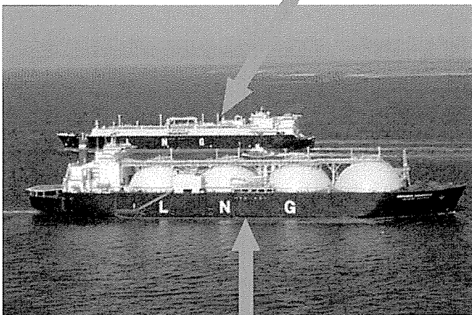
Self supporting tank: Kvaerner Moss
